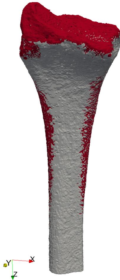
Figure 7.19: Bending radius test with elasto-plastic material properties. Yielded elements are shown in red.
